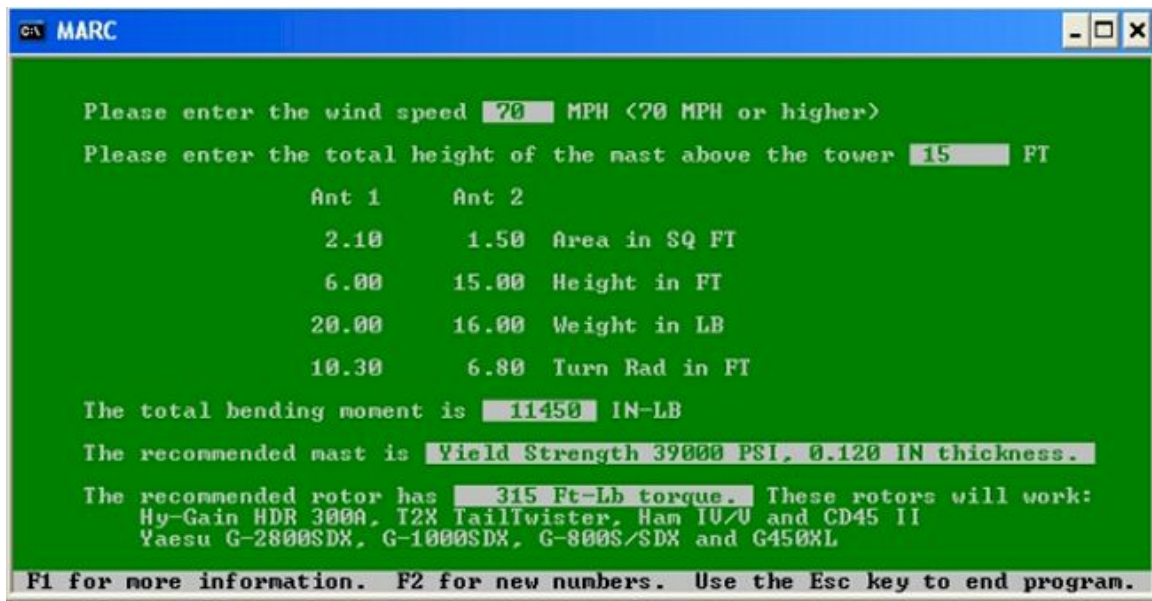
Fig. 3. After entering data from my failed system into highlighted fields in vintage DOS style, I got the results shown in the screen capture. As you can see, the bending moment I should have allowed for, according to MARC, was 11,450 inch-pounds. A 2-inch mast with a 1/8-inch wall thickness, and yield strength of 39,000 PSI would have met the requirements.
