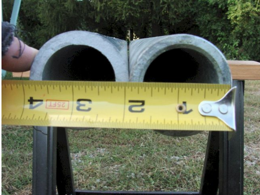
This shows the wall thickness of 0.25 in., and the OD of 2 in. Beefy!
