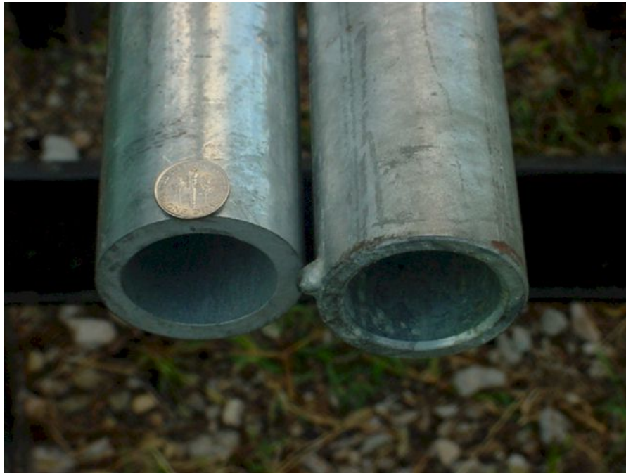
Here's an oblique view of the ends, with a US dime sitting on the left tube for scale. Note the galvanizing "pimple" on the one on the left. Not too esthetically pleasing, but it won't affect the function.
