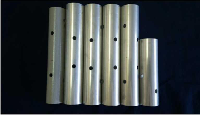
Coupling inserts. Leftmost is the fiberglass insulator for the top of the base mast section. Short one is 4-3/4" (120 mm) for the top section. The rest are 7-1/8" (182 mm) long.
