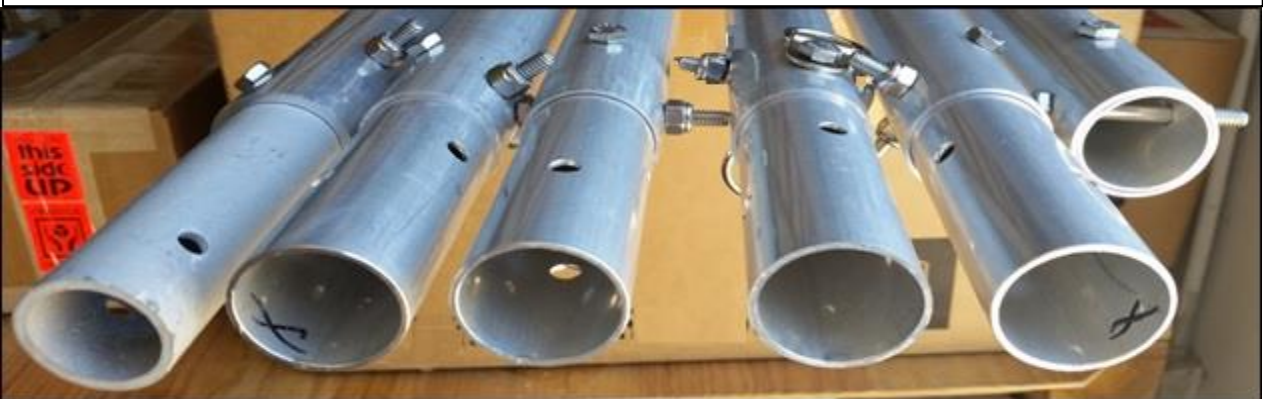
Mast sections with its coupling inserts attached at their tops. Note the two tie down "D" rings for guy ropes at the top of the fourth section (SAL-30 Mark II only) and the shortest insert to reinforce the tubing at the connection point at the antenna apex, it is flush with the top section's end.
