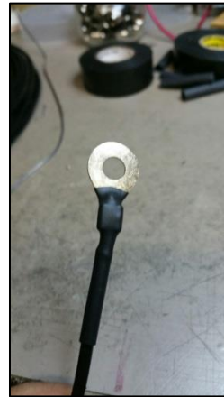
Solder lug and wire connection protected with shrink tubing. Rubber tape can be used as well.
