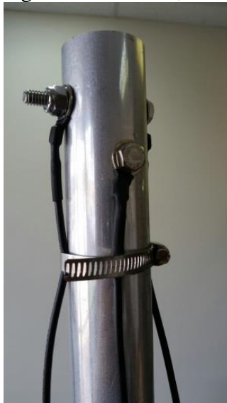
The four top ends of the wires connected to the apex of the antenna, and the hose clamp used to relieve the tension from the connection lugs.
