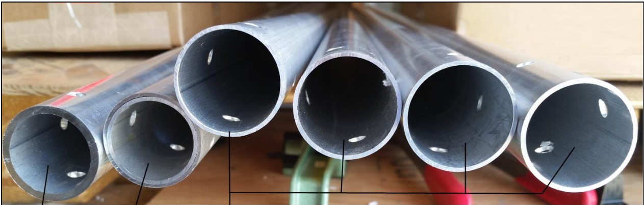
Top of base pipe, bottom has no holes for bolts. It is double wall Second section bottom, the bottom has a riveted insert to match the wall thickness of base section and accommodate the insulator that connects base and second section All the other four sections (SAL-30 Mark II) are the same and there is no difference between their top and bottom. All will have coupling insert with the following section, except the top section which has a shorter insert to reinforce the top connection points on the three SAL - Mark II models. SAL-20 Mark II: Two of these sections and the bottom and second section (4' + 6' + 6' + 6'). SAL-12 Mark II: One of these sections and the bottom and second section (4' + 6' + 6').
