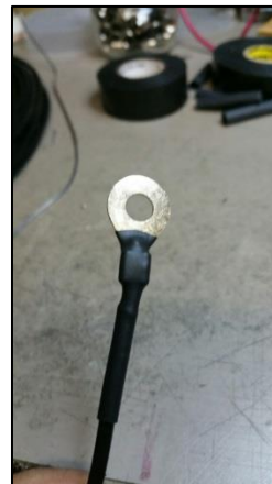
Solder lug and wire connection protected with shrink tubing. Rubber tape can be used as well.
