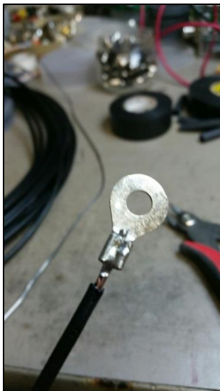
Crimped and soldered lug.
