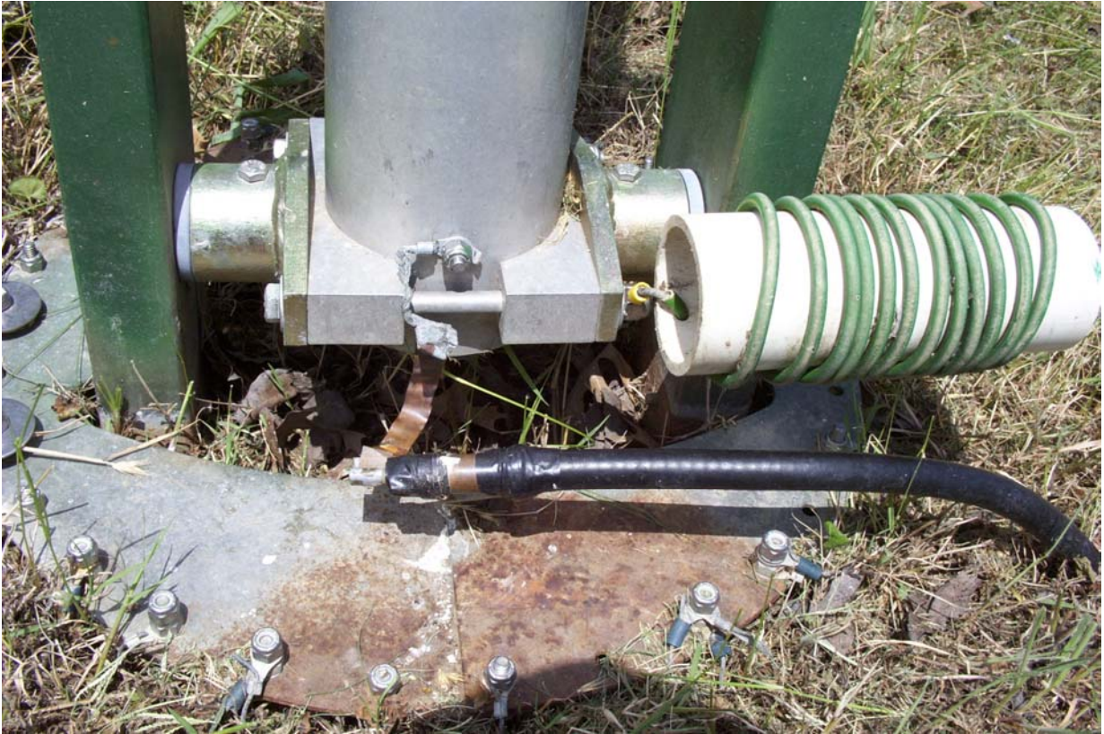
Fig 7 – Inductor attached to the insulated vertical element and grounded at far end (not shown in picture).
