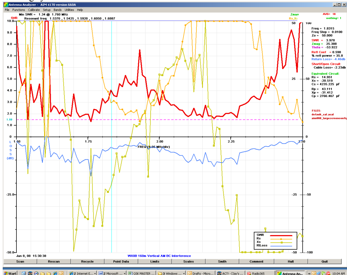
Fig 3 – plot of antenna from 1.5 to 2.5 MHz, AM broadcast is making the measurement useless.
