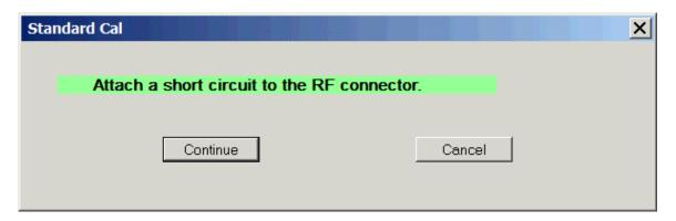
Attach the connector with an internal short circuit (this is included with the AIM, it has a green label and is labeled "short").
