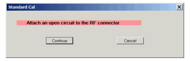
**Replace** the short circuit with an **open connector** (this has a red label and is included with the AIM) and then click **Continue**.
