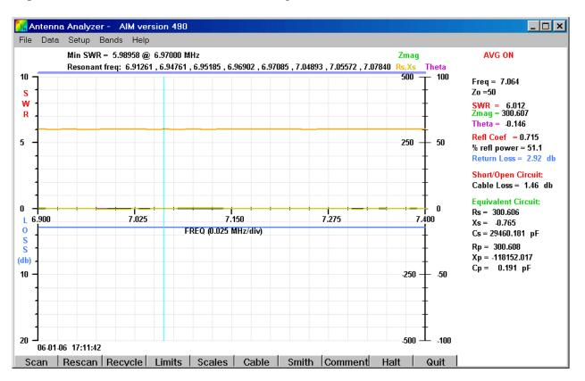
Scan using a 301 ohm resistor for a test load.
