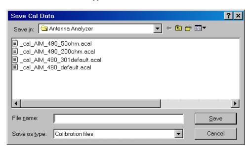
Enter the name of the calibration file and click "Save". There is no restriction on the name of the cal data file. It's extension is automatically set to .acal ("analyzer cal"). Any of these cal files can be recalled latter using the menu option "File" → Load Cal File.
