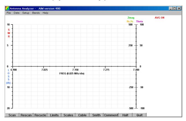
When the AIM hardware is present, it must be turned on **before** the PC program is launched.
