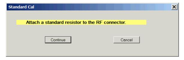
After taking several reading of the open connector, the program will prompt for the standard resistor with a value between 50 ohms and 500 ohms. This resistor typically has a yellow label and it's included with the AIM kit. If you want to cal with a different resistor, the exact value is not critical. Enter the value you measured with a digital ohmmeter and click Continue.
