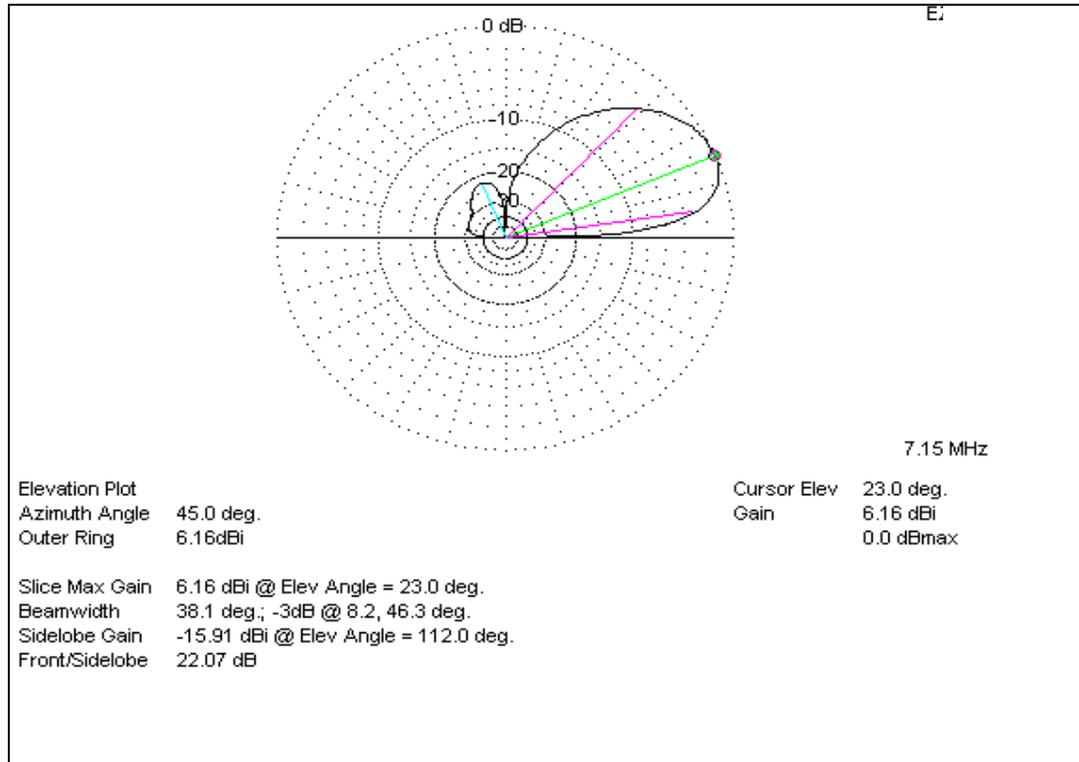
**We have increased the gain by 0.66 dB and the front to back ratio by 6 dB or more!**
