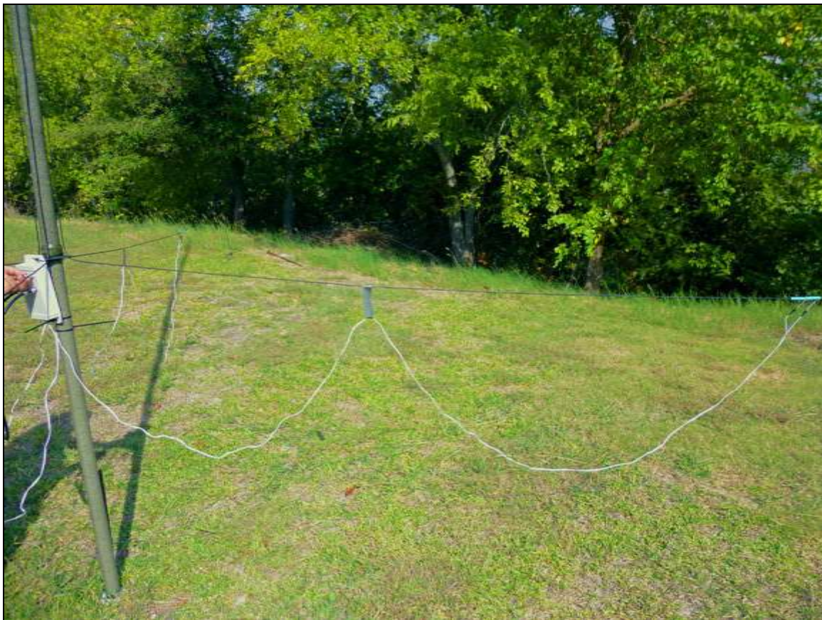
Coupler's transmission line is kept clear of ground and other loop transmission lines
