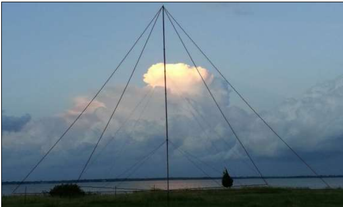
View of the SAL-30 antenna. The loops' wires have been edited thicker for clarity. The thin lines are the guying ropes.
