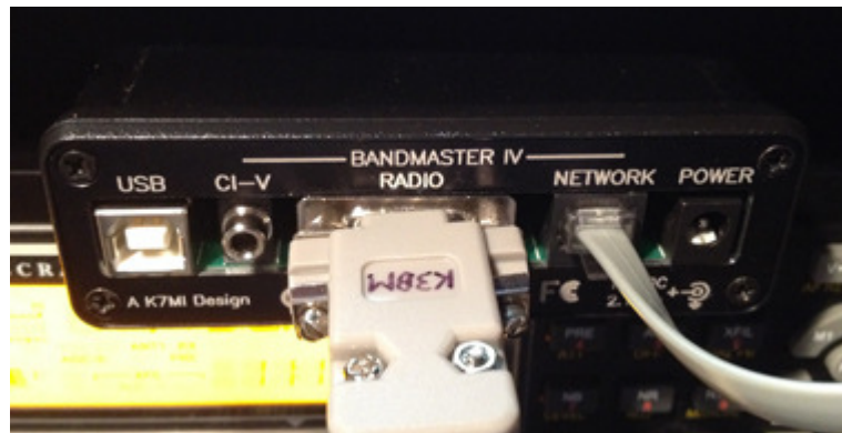
Figure 1 - Rear View (Showing a K3BM [Elecraft K3 to BandMaster] cable and an RJ-14 network cable connected)
