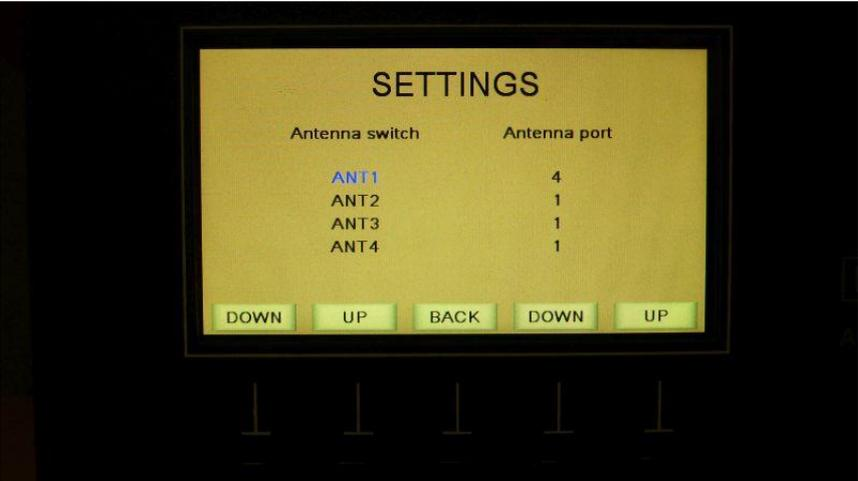
With the **DOWN** and **UP** buttons on the left side it is possible to select the individual antenna positions, and with the **DOWN** and **UP** buttons on the right side it is possible to select the corresponding ports on the external antenna switch. If all 4 antennas have been set, then it is possible to return to the previous menu point with the **BACK** button.
