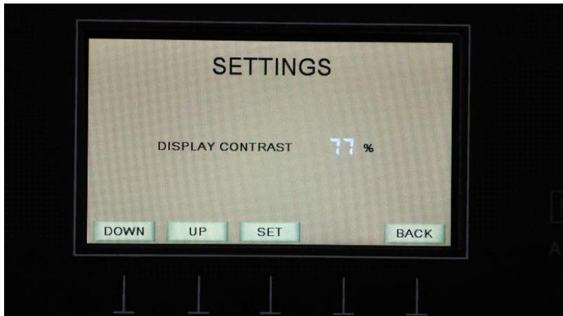
With the **DOWN** and **UP** buttons it is possible to set the brightness of the display. The value set is placed in the memory with the **SET** button, or with the **BACK** button it is possible to return to the settings menu. In this case the brightness value set is not put in the memory.
