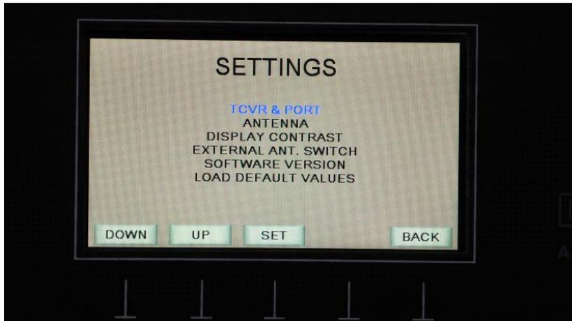
**TCVR & PORT** – selects the radio type and the parameters for the serial port
