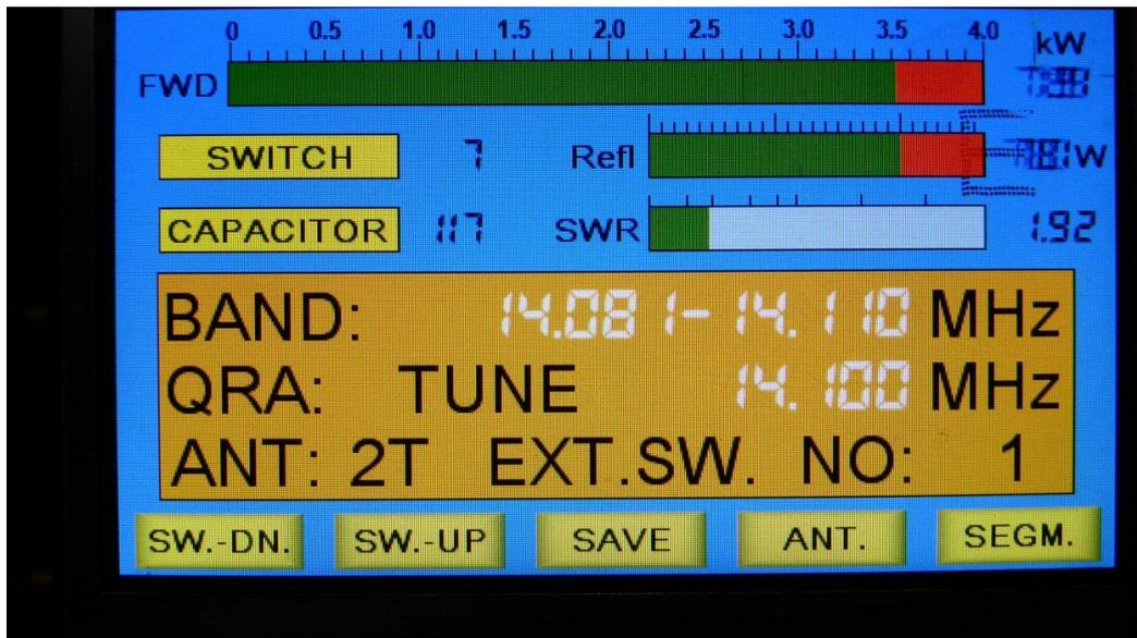
After pressing the **TUNE** button it is possible to tune the individual antennas
