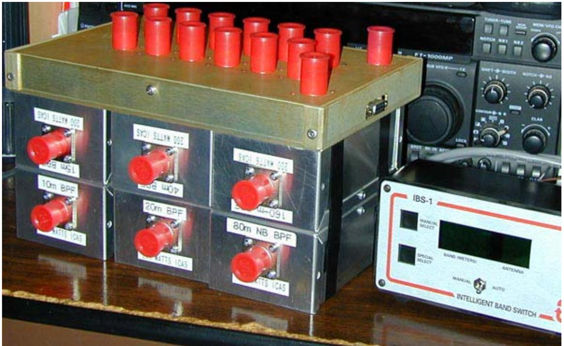
The above picture shows the FM-6 on top of 6 W3NQN Filters, which are strapped together. The coaxial cables will be routed next around from the FM-6 to each individual filters input and output connector.
