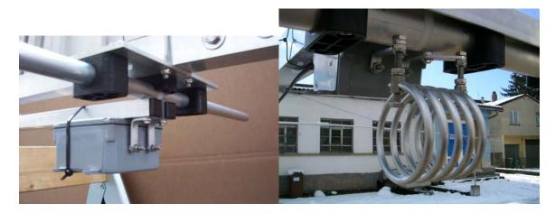
The bracket for the balun is available from Array Solutions or from Optibeam in Europe. If you use a cable tie, clip it clean and place a few wraps of tape over it to keep UV off the cable tie.
