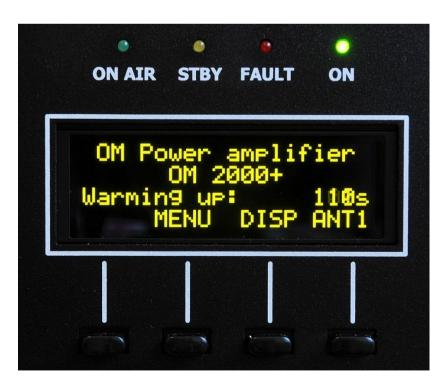
**S1 S2 S3 S4**  **ON AIR** - Transmitting mode LED
