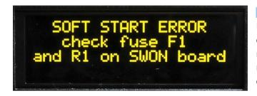
If resistor R1 or fuse F3 is damaged, safety circuit stops starting of the PA and fault message appears on the display. It is necessary to replace the damaged component.
