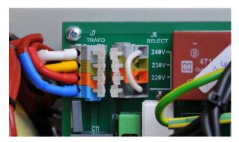
Use flat screwdriver or finger and press carefully the white stick to release contact and move upper end of the white jumper to the proper position, if necessary.
