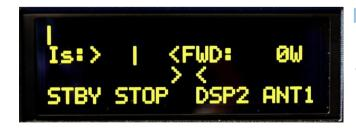
PA is in the operation mode. After **TUNE** button (S2) was pressed, it changes its function. Now **STOP** is blinking.
