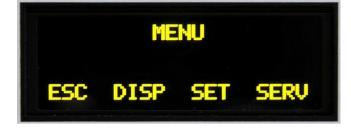
After pressing **MENU** (S2) S1–S4 buttons changed their functions. To edit display parameters, press **DISP** button.
