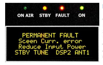
This is the situation, when problem with high Input power persists. Safety circuits reacted 3 times, and then switched PA to STBY mode. Permanent fault appears.
