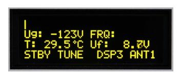
Check all connections again. Set BAND selector, TUNE and LOAD capacitors according to TCVR parameters and delivered tuning table (see next part for more details). Apply **low input power** and press PTT. Check Analog wattmeter first. Try to tune PA for maximum output power and minimum SWR.
