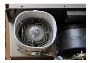
Detailed view on the tube and blower area. Antenna switch (above) is installed inside the metal box.
