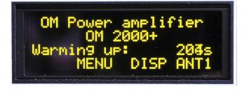
Warming time takes abt. 210 seconds. It is possible to enter **MENU** during this time, but with limited possibilities (display settings can be changed, for example).
