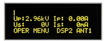
Changing of **DSP** allows user to watch couple of basic parameters of the PA in operation mode without input RF signal. Notice: These are three default display settings (software version 6.1.)
