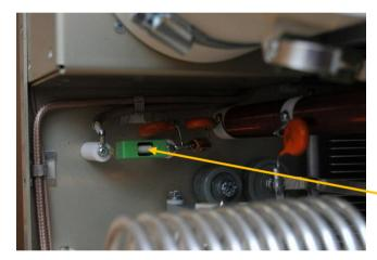
One special fuse is used in the model OM2000+. In the case of an accidental discharges in the tube this fuse saves HV supply circuits.
