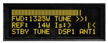
Two of important information is visible – screen current increased, but still is within the allowed limits. Turn LOAD knob slightly in arrows direction to get TUNE indicator between arrows.
