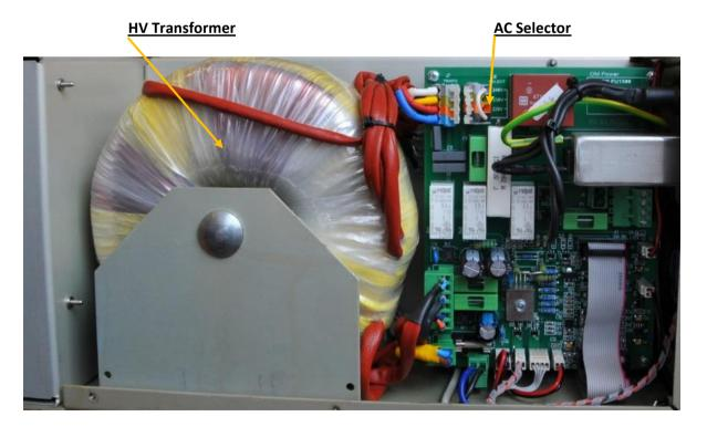
Remove the upper lid first. On the right side of the PA, next to the HV transformer there are two PCBs mounted. On the left upper side of the front (Switch-ON) board connector J6 is located.
