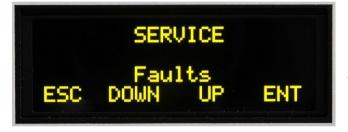
Use **UP** or **DOWN** button to select Faults. Press **ENT** to see fault numbers or letters (see the table in chapter 6).
