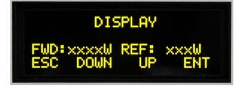
Go **UP** or **DOWN** to select desired parameter. Press **ENT** to confirm selection.
