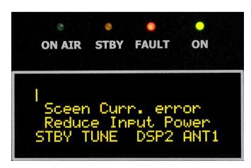
An example shows situation when Input power is too high. By pressing PTT safety circuit will react quickly, error message appears and FAULT LED starts blinking. In this case screen current exceeds limited value (60mA).
