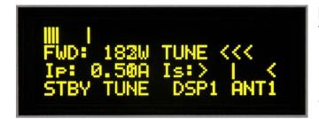
This is not an optimal result, TUNE indicator must go between both arrows. Use **TUNE** knob **to get maximum output power** and LOAD knob **to get indicator between arrows.**
