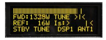
Display indicates **correct tuning** of the Power amplifier.
