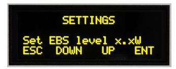
Use **UP** or **DOWN** button to select EBS level parameter. Press **ENT** to enter EBS level settings.
