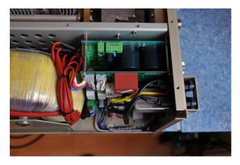
3 kVA toroidal transformer is visible on the left side. Switch-ON board is in the front, Power supply board behind it.
