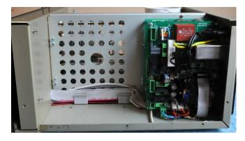
Weight of the PA was distributed (transformer has 12 kg, rest of the PA has cca 12 kg, too).
