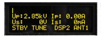
Without RF power the plate voltage is 2.85 kV. Check the heating voltage, too. If it is below 8.5 V, this indicates the need to change AC selector position one step down (for example from 230 to 220 VAC).
