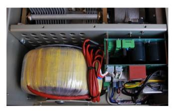
Watch the released terminals, when moving the transformer!
