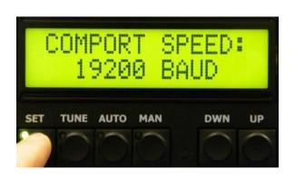
Baud rate for TCVR – PA communication is shown on the LCD display.
