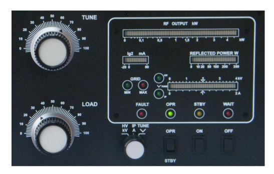
**TUNE -** Anode capacitor for tuning, tuning of higher frequencies to "0", lower frequencies to "100".
