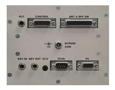
KEY IN KEY OUT RCA Phono - Input signal PTT switching voltage / current 5V/2 mA) RCA Phono - Output signal PTT (maximum switching of 30V/50mA)
