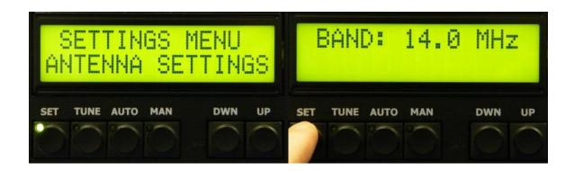
Then select how many antennas you want per current band (1 or 2) and always confirm your selection by pressing SET. The by scrolling UP / DWN you assign which PORT is used on your external antennas switch for this particular antennas. (ANT 1 ON PORT 01)
