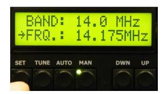
To enter Manual mode of the PA please press MAN. By pressing MAN repeatedly you select BAND and band segment. You can control the segment or band by scrolling the UP / DWN buttons.
