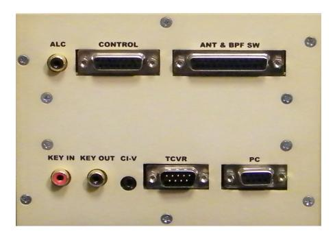
KEY IN KEY OUT RCA Phono - Input signal PTT switching voltage / current 5V /2 mA) RCA Phono - Output signal PTT (maximum switching of 30V / 50mA)
