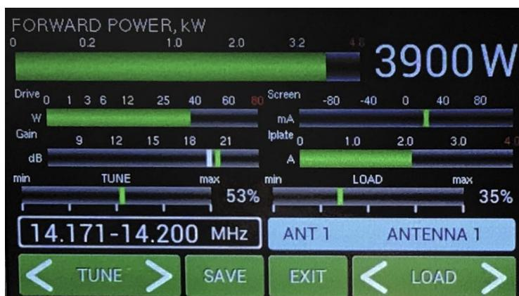
Press **MENU, M-TUNE)** and make the manual adjustment.
