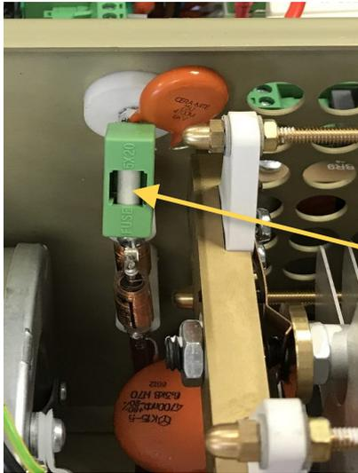
One special fuse, filled with sand, is used in the model OM40001A. In the case of an accidental discharges or short within the tube this fuse (4 Amps fast, filled with sand) saves the HV supply circuits.
