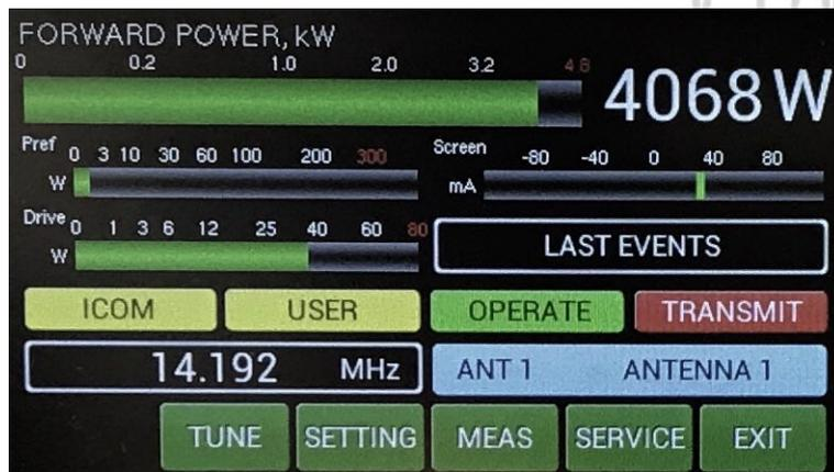
We can now see a new small yellow **USER** window in the touch screen display. **USER** means that we used the M-TUNE feature to optimize the PA adjustment.
