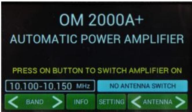
Switch ON the power amplifier using the front panel green ON switch.
