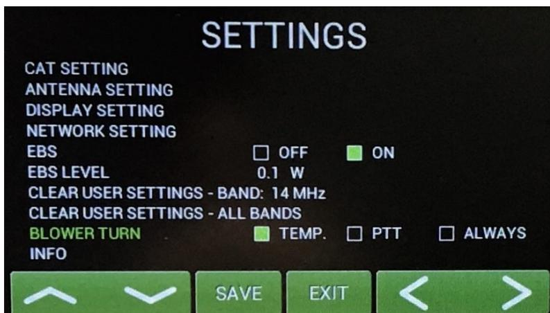
In the next line you can define working mode of the blower. In the first mode speed depends on the PA temperature (**TEMP**), In **PTT** mode the speed increases to maximum, and the **ALLWAYS** mode means maximum speed all the time during PA operation (recommended for DIGI modes).
