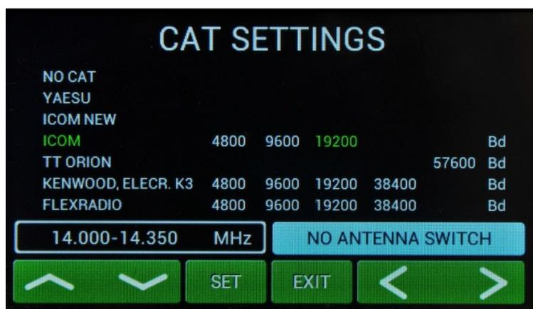
If you choose **YAESU** or **ICOM NEW**, after **SET** pressing you will go to deeper level which allows you to select specific type of TCVR.
