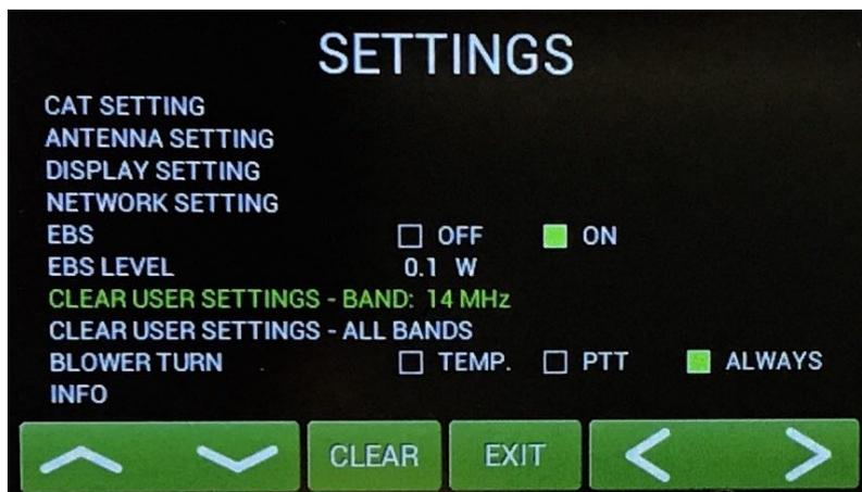
The next two settings allow deletion of the manual user settings of the amplifier tunings for a single band or for all bands.
