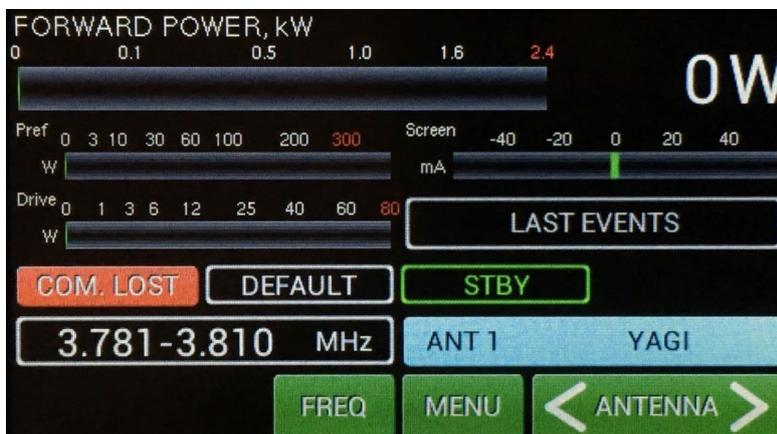
**FREQ** button has two functions. It allows displaying the working frequency or active band segment.
