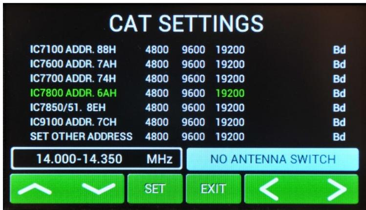
You selected IC7800 addr.6AH and 19200 Bd. Press **SET** to write to the memory, then press **EXIT** to go back to the **SETTINGS** possibilities.
