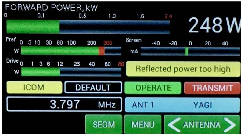
This is an example from a previous attempt at transmitting when the antenna was disconnected from the PA .
