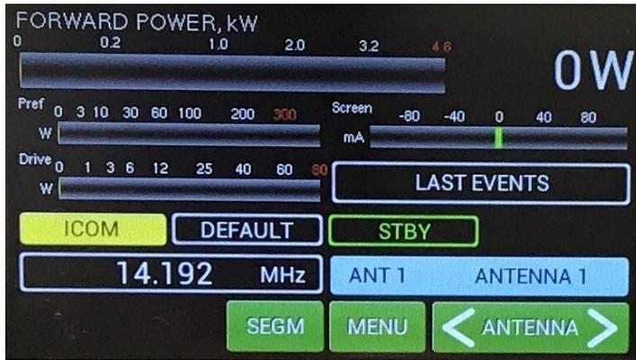
The **Menu display** allows the user to go deeper into the SETTINGS mode, MEASuring mode or -SERVICE mode.
