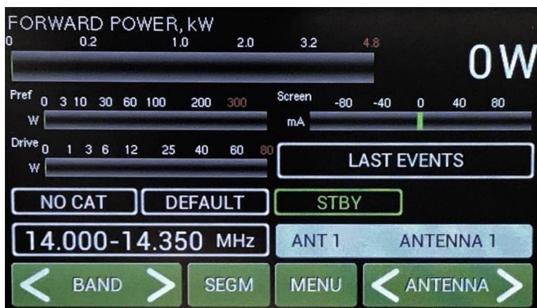
After heating is completed, the PA will light the **STBY** mode indicator and this **Main display** will appear.
