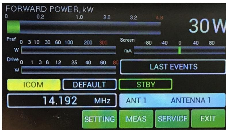
Measured driving power is 30 Watts.
