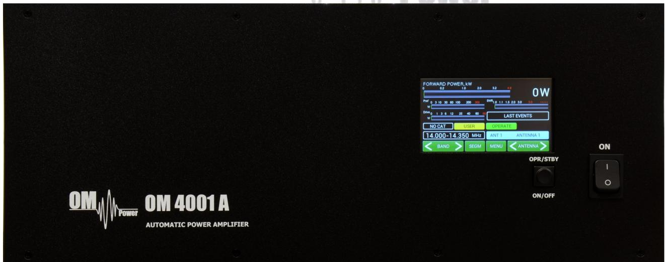
**ON - Main Switch.** After turning ON, a small 12V APU for logic, protection circuits and the display will be activated. High voltage and RF circuits are still OFF.
