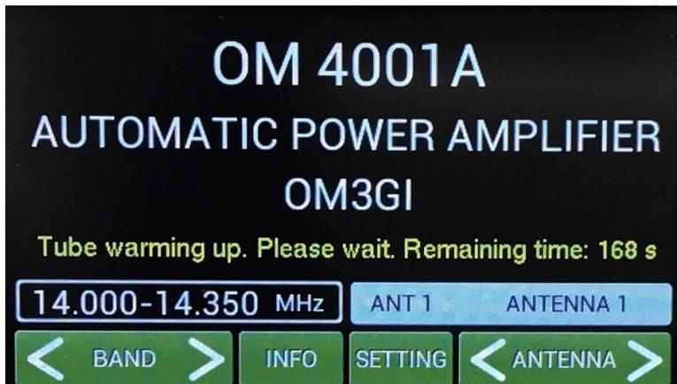
The “Tube Heating Timer” is visible on the display. Wait until the required 180 seconds is complete before placing the amplifier in OPERATE Mode.
