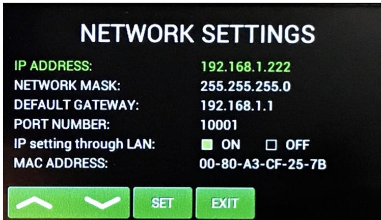
Here the user has the option to set IP Address, Network mask, Default gateway, Port number.
