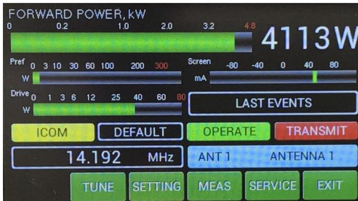
Output power is 4113W, reflected power about 1W and screen current is about +50 mA.
