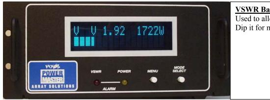
VSWR Bargraph Mode Used to allow easy adjustment of a tuner for minimum VSWR. Dip it for minimum VSWR.
