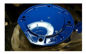
Align the bottom lid center holes with the metal holder screw pylons and secure with the two screws previously removed. Then align the lid with the markings and secure it with the remaining screws.
