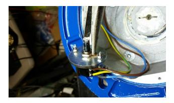
Remove the potentiometer from the metal holder by unscrewing the nut and its washer.
