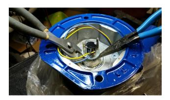
If the potentiometer and metal holder assembly do not come out easily pulling it by hand, use suitable tools as levers on both sides of the potentiometer assembly to take it out. Levers most exert symmetric upward force to avoid breaking the potentiometer shaft. The shaft is made of plastic most of the time.
