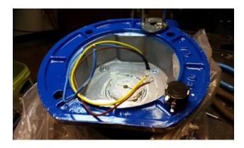
Desolder or cut the wires from the potentiometer.
