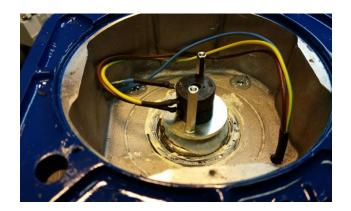
Solder the cables in the right order. Put the potentiometer assembly in place.
