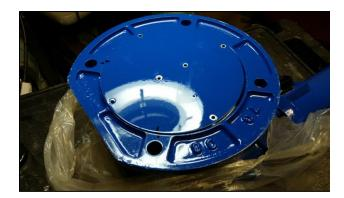
Make one or two reference markings to remember the position of the bottom lid, before removing it.
