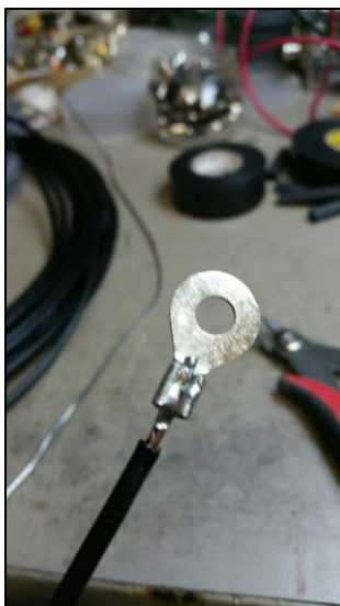
Crimped and soldered lug.
