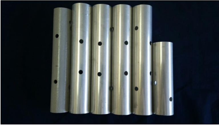
Coupling inserts. Leftmost is the fiberglass insulator for the top of the base mast section. Short one is 4-3/4" (120 mm) for the top section. The rest are 7-1/8" (182 mm) long. NOTE: SHORT COUPLER MAY BE PREINSTALLED IN TOP SECTION.
