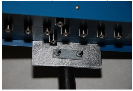
The location for the StackMatch II Plus can be physically between the antennas although most prefer to mount the StackMatch at the base of the tower. If you choose to do this, remember that you still must cut equal lengths of feedline for each antenna. Note: the lower antenna cable will be extra long, so plan to coil it up loosely and use ty-wraps to keep it neat at the base of your tower.
