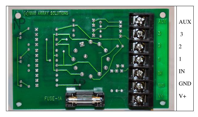
Make a chart of your wire colors so you can connect the correct wires in the StackMatch II Plus relay box. Use the Ty-Wrap<sup>TM</sup> supplied to secure the cable from pulling out of the box.
