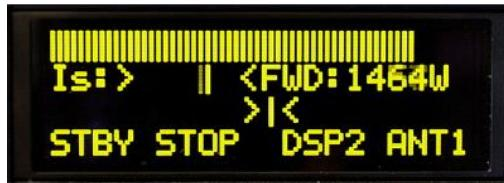
11. Stop transmitting and press the S2 button (under the blinking STOP on the screen) to get the amplifier out of the TUNE mode. The screen will show “TUNE” above the S2 button. The amplifier is tuned and ready to operate.
