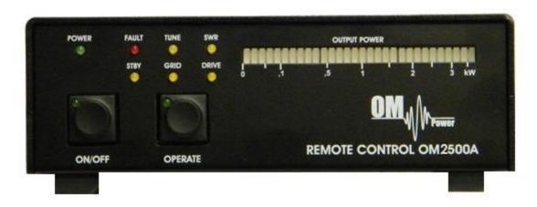
ON / OFF - Standard ON / OFF switch. On state is indicated by green LED on the switch
