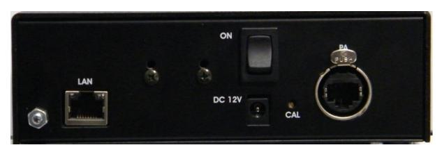
LAN - Standard RJ45 connector - LAN Interface for remote access
