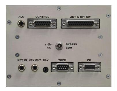
**KEY IN** RCA Phono - Input signal PTT switching voltage / current 5V /2 mA)
