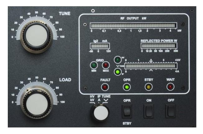
**TUNE** Anode capacitor for tuning, tuning of higher frequencies to "0", lower
